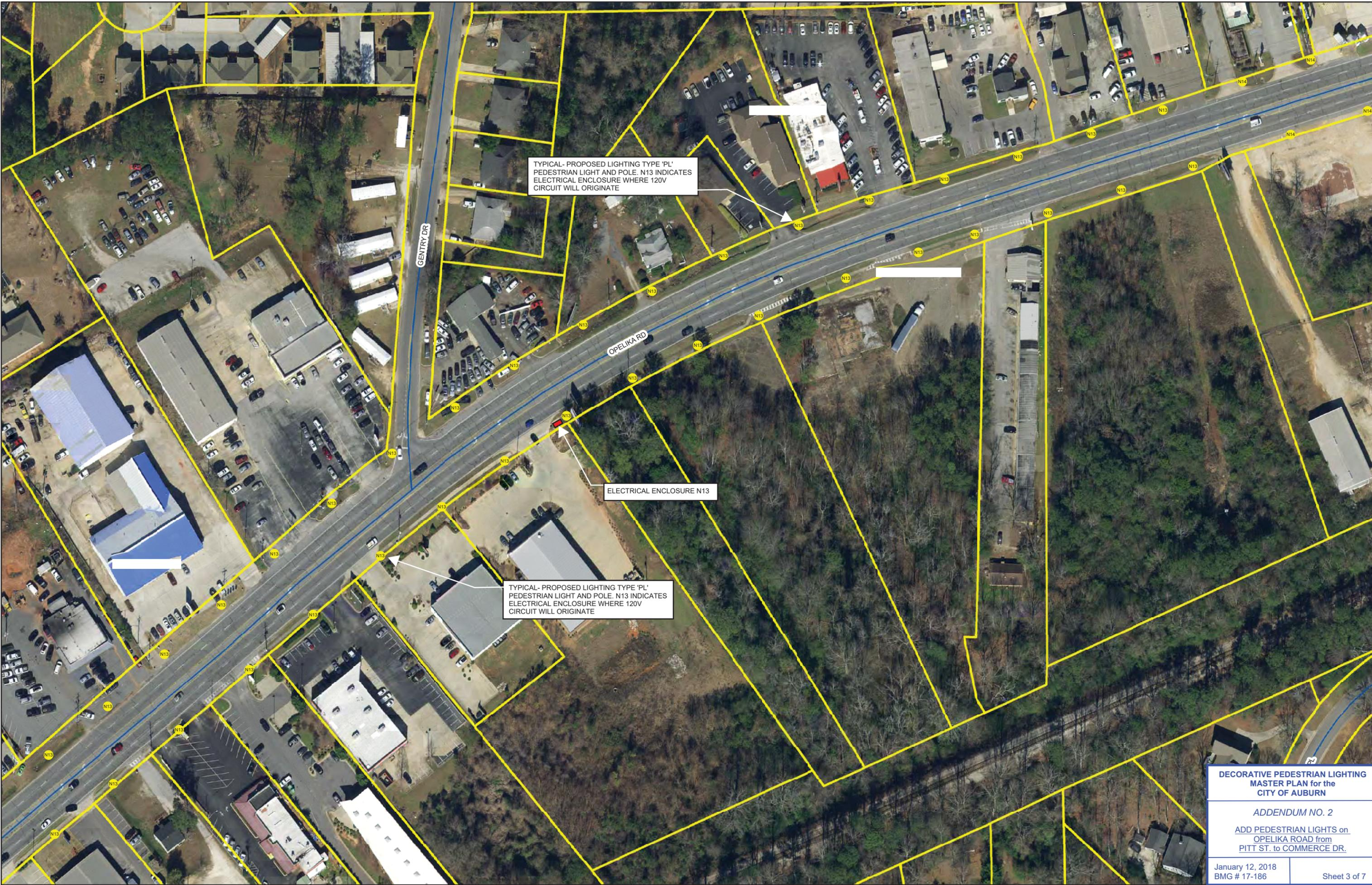
TYPICAL- PROPOSED LIGHTING TYPE 'PL' PEDESTRIAN LIGHT AND POLE. N13 INDICATES ELECTRICAL ENCLOSURE WHERE 120V CIRCUIT WILL ORIGINATE
