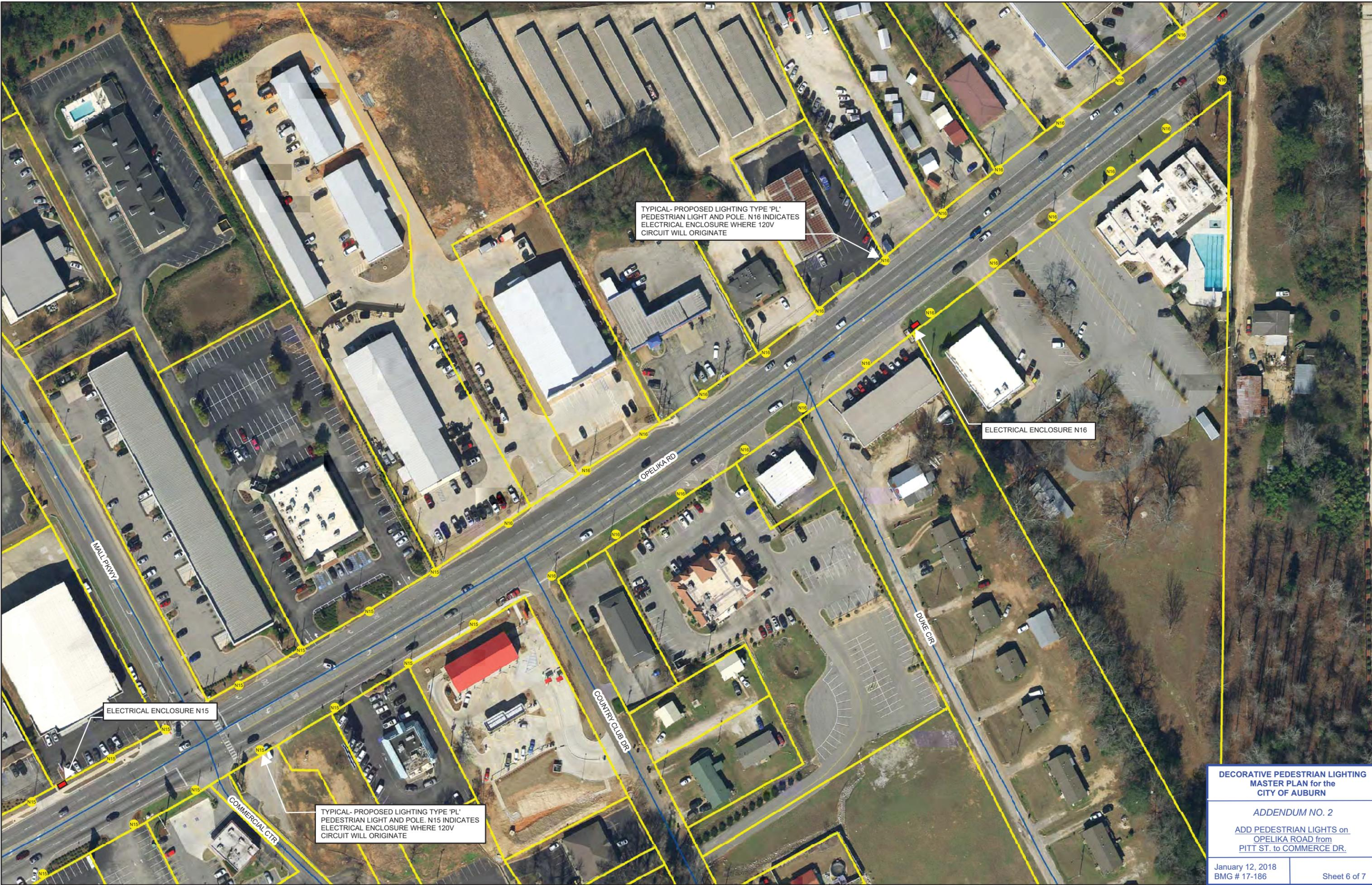
TYPICAL- PROPOSED LIGHTING TYPE 'PL' PEDESTRIAN LIGHT AND POLE. N16 INDICATES ELECTRICAL ENCLOSURE WHERE 120V CIRCUIT WILL ORIGINATE
