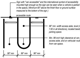
96" min. width access aisle, level (max. slope 1:50 in all directions), located beside the van
