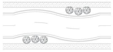
FIGURE 3 Example of a Chicane
