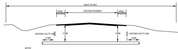
1. CASING SHOULD EXTEND AT LEAST 5' BEYOND EXISTING UTILITIES OR EDGE OF PAVEMENT, WHICHEVER IS GREATER.
