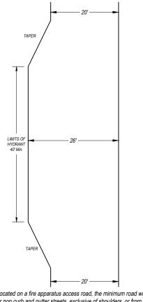
When a fire hydrant is located on a fire apparatus access road, the minimum road width shall be 26 feet from EP - EP for non curb and gutter streets, exclusive of shoulders, or from face of curb face of curb for curb and gutter streets, for at least 40 feet at the hydrant.
