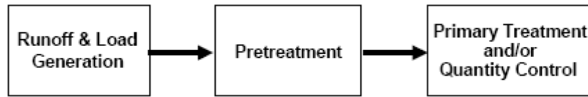
FIGURE 4-34 Generalized Stormwater Treatment Train
