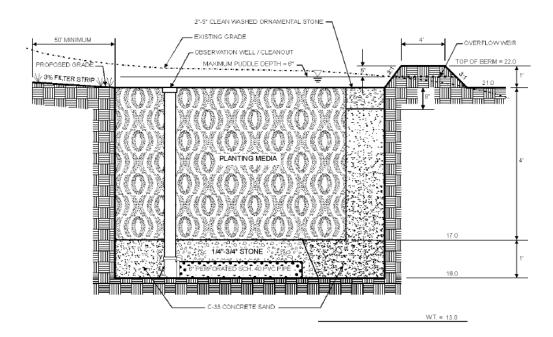
FIGURE 4-7 Bioretention Facility Typical Section Source: GSMM (2001)
