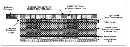
Figure 3.3.8-2 Modular Porous Paver System Section
