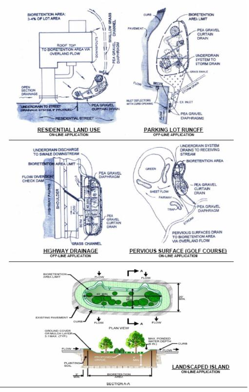
FIGURE 4-4 Bioretention Applications Source: GSMM (2001)
