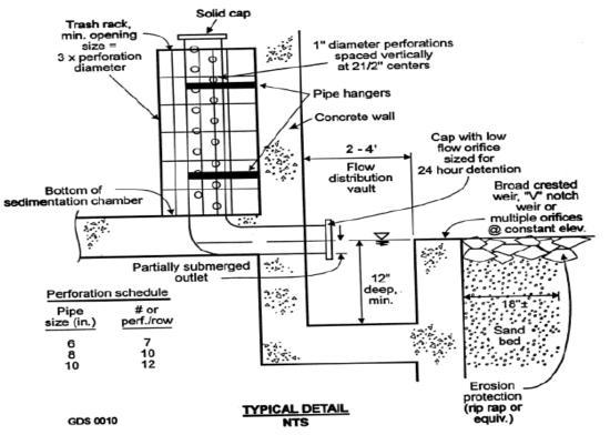
FIGURE 4-23 Detail for a Surface Sand Filter Perforated Standpipe Source: GSMM (2001)
