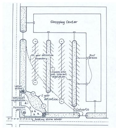
FIGURE 4-38 Example Treatment Train–Commercial Development Source: NIPC (2000)
