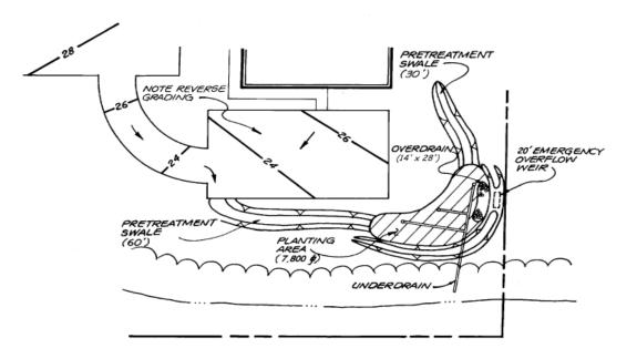
FIGURE 4-6 Bioretention Facility Layout Source: GSMM (2001)
