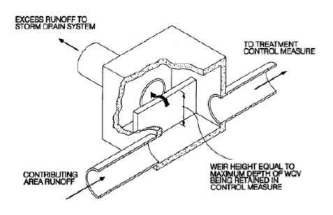
FIGURE 4-31 Pipe Interceptor Diversion Structure Source: City of Sacramento (2000)
