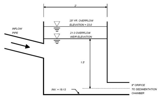
FIGURE 4-26 Flow Diversion Structure Source: GSMM (2001)
