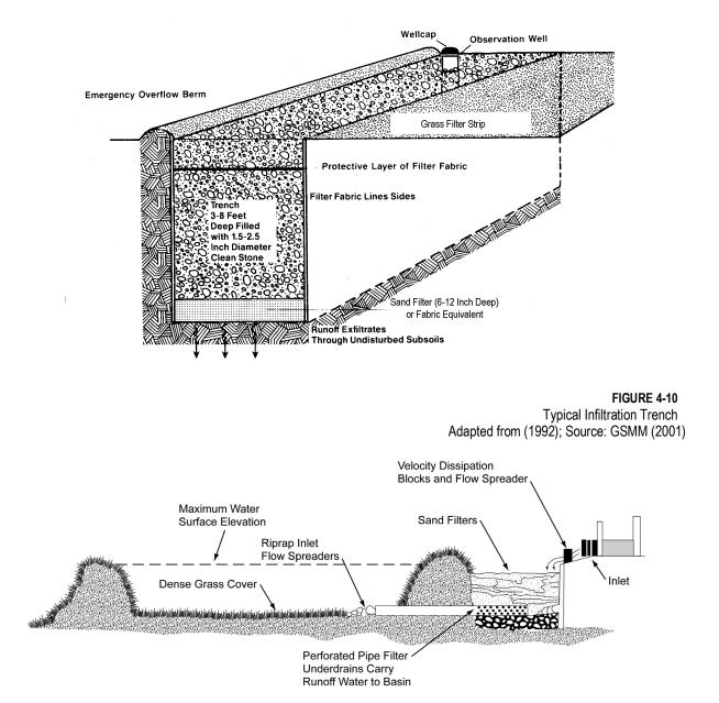
FIGURE 4-11 Typical Infiltration Basin with Sand Filter Source: GSMM (2001)
