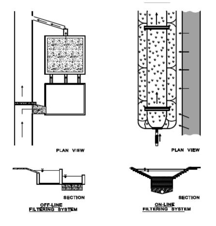
FIGURE 4-30 Example of Online versus Offline Structural Controls Source: CWP (1996)
