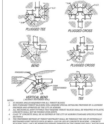
BLOCKING SHALL ONLY BE PERMITTED WHERE APPROVED BY THE AWWB AND SHALL NOT BE USED BIOCONJUNCTION WITH MEGA-LUG RESTRAINTS. THE APPROPRIATE LENGTH OF RESTRAINT SHALL BE CALCULATED IN ACCORDANCE WITH THE MANUFACTURERS RECOMMENDATIONS.
