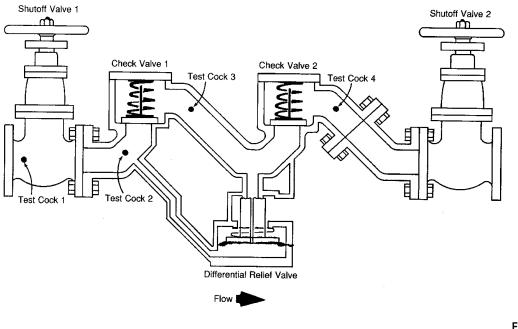
FIGURE 2-3 Reduced Pressure Backflow Assembly (RPBA) AWWA Manual M14, Backflow Prevention and Cross-Connection Control
