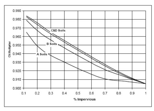
FIGURE 4-39 Curve Number Adjustment Factor
