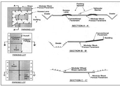
FIGURE 4-18 Typical Permeable Paver Design
