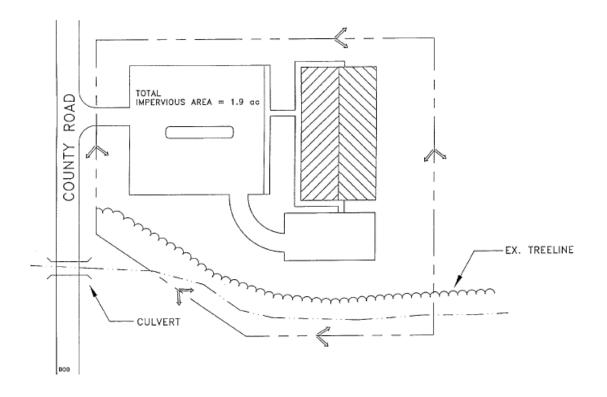
FIGURE 4-5 Bioretention Example Site Plan Source: GSMM (2001)
