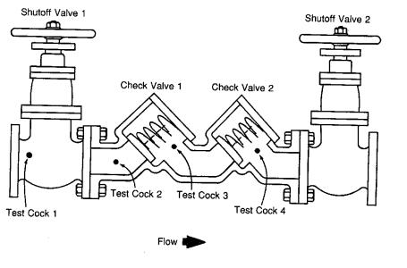
FIGURE 2-2 Double Check Backflow Assembly (DCBA) AWWA Manual M14, Backflow Prevention and Cross-Connection Control
