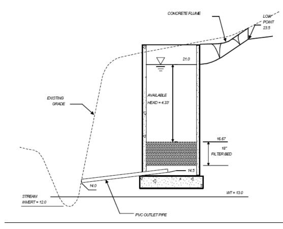
FIGURE 4-25 Head Diagram Source: GSMM (2001)
