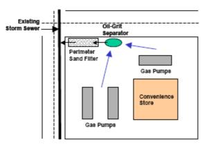
FIGURE 4-37 Example Treatment Train–Commercial Development
