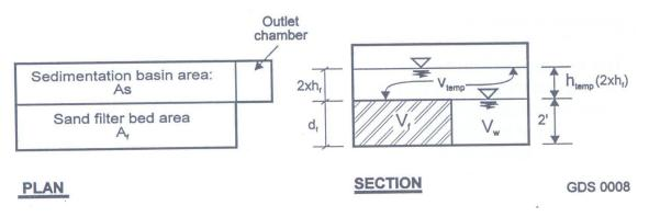
FIGURE 4-21 Perimeter or Closed Sand Filter Volumes Source: Claytor and Schueler (1996)
