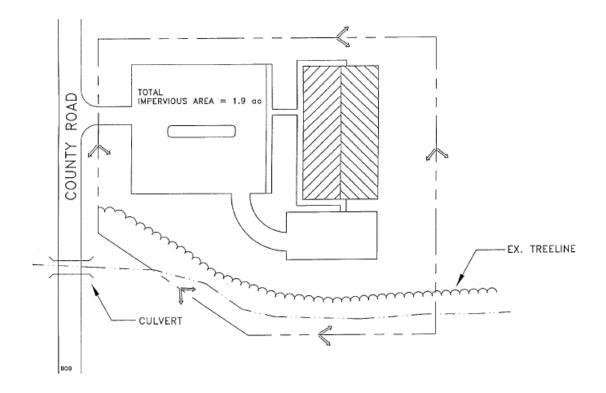
FIGURE 4-12 Infiltration Trench Example Site Plan Source: GSMM (2001)
