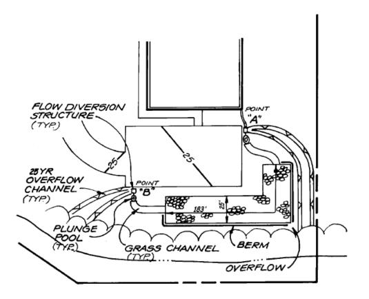
FIGURE 4-13 Infiltration Trench Site Plan Source: GSMM (2001)
