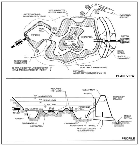
Note: Channel Protection Volume (CPv) shown in Figure 4-2 is not used in Auburn. The weir invert elevation at the CPv elevation should be set to meet the City's discharge criteria, as detailed in the City of Auburn *Stormwater Management Manual*.
