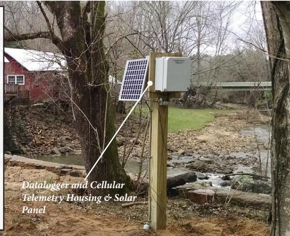
*Datalogger and Cellular Telemetry Housing & Solar Panel*
