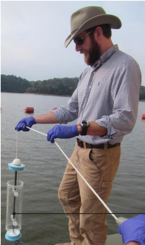
Kemmerer Sampler Used for Obtaining Samples at Specified Depths in Lake Ogletree
