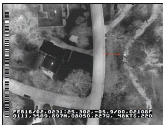
Figure 72: Aerial thermography showing sewage leak
