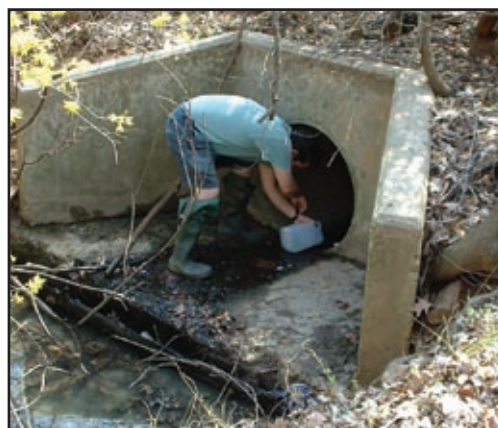
Figure 30: Measuring flow (as volume per time)
