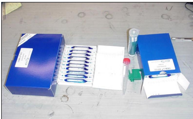
Figure F3.1: CHEMetrics detergent test kit components
